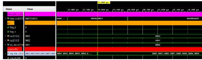
Figure 11: Register File Contents After Second SUB
