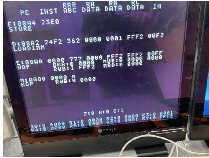
Figure 13: Overflow Test (0 = error) on Console Display
